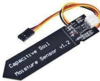
Gambar 8 Soil Moisture Sensor
