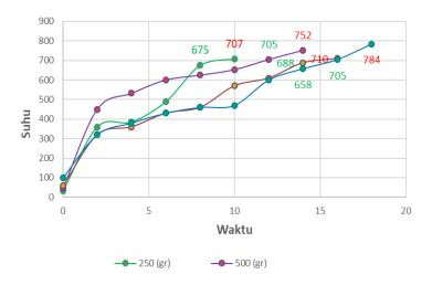
Figure 4. Graph of Melting temperature and time at volume 250, 500, 750 and 1000 grams of waste aluminum metal
