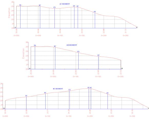
Figure 6. Ground Level Surface Along with CL of Horizontal Alignment
