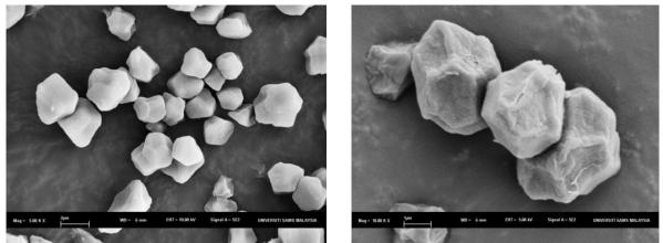
Figure 3. Scanning electron micrographs of *D. hispida* starch granules. Left, 5000×; Right, 10000×
