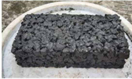
Figure 7. Moulding Porous Paving
