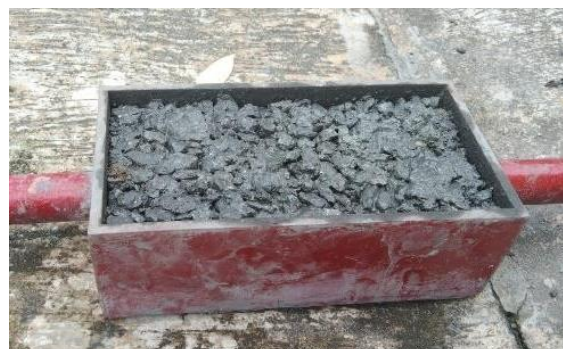
Figure 6. Moulding Porous Paving
