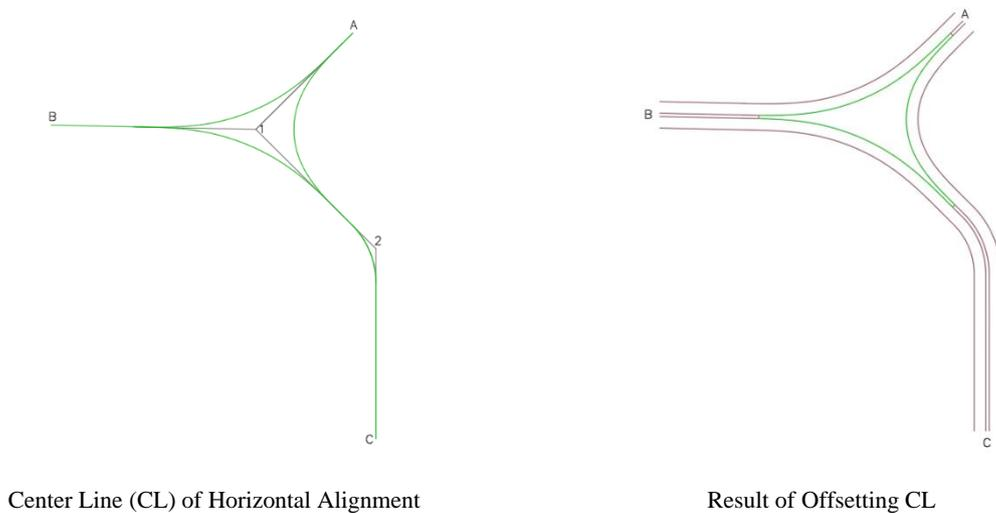
**Figure 5.** Horizontal Alignment Plan
