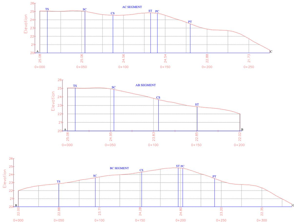
**Figure 6.** Ground Level Surface Along with CL of Horizontal Alignment
